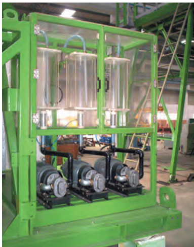
Admixture weighing system for chemical additives.
