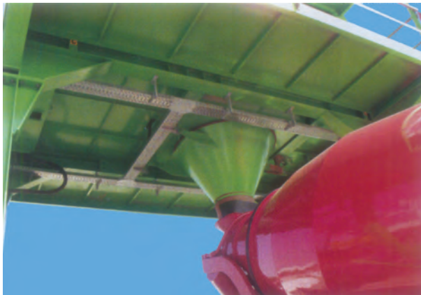
The mixer discharge for filling truck mixers.
