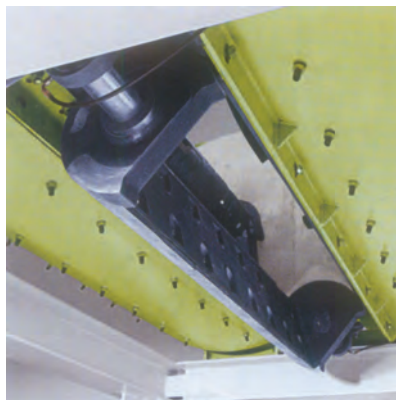
The discharge gate.
