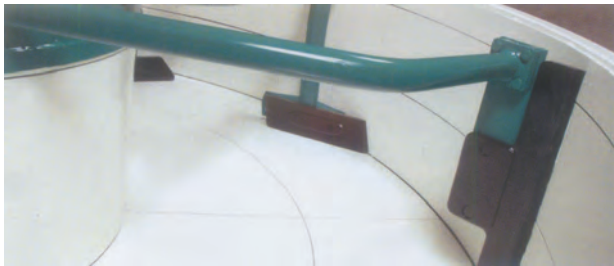
Pictures top left and right : inner and outer scraper support mixing and discharging effect.
