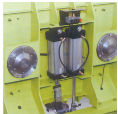
The pneumatic discharge gate operation
