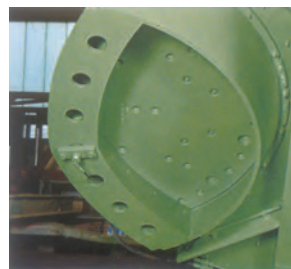
Large-dimensioned mixer discharge with hydraulically actuated sliding gate for fast discharging.
